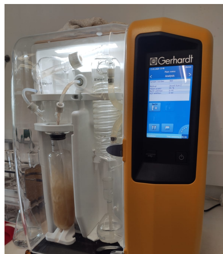
Figure 2: Distillation systems from kjeldahl analysis (Model: Gerhardt VAPODEST, image took at ISA University)
