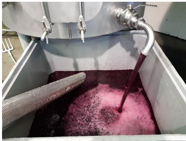
Figure 23 - Bleed a fermented tank to be able to press the masses (author's photo)
