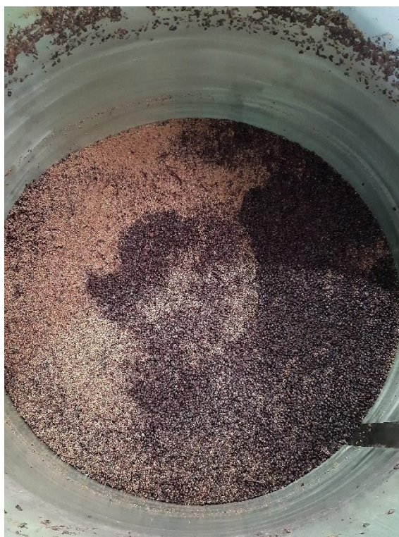
Figure 24 -Inside a tank after bleeding, by the mark in the top it's possible to see where it was before (author's photo)
