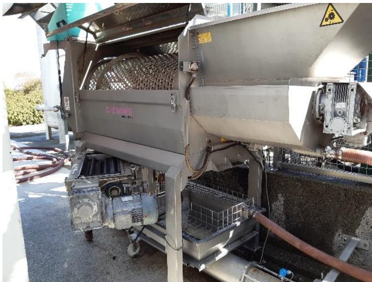
Figure 16 - Destemmer/Crusher where it's possible to see the destemmer drum and below the Crusher (author's photo)
