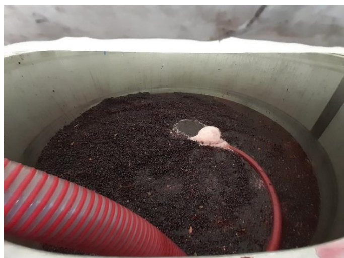
Figure 21 - Pump over during maceration (author's photo)
