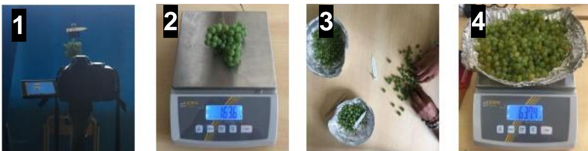
Figure 9 The detailed measurement performed in the laboratory on 2019, from the left to the right the blue background used to take the pictures of the bunches, the scale used to weight the bunches, the berries separation and the weight of the berries.
