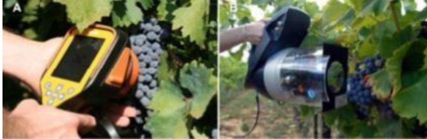
Figure 1. Spectron (A) and Multiplex (B) hand-device sensors for quality of grape (Source: Matese and Di Gennaro, 2015).
