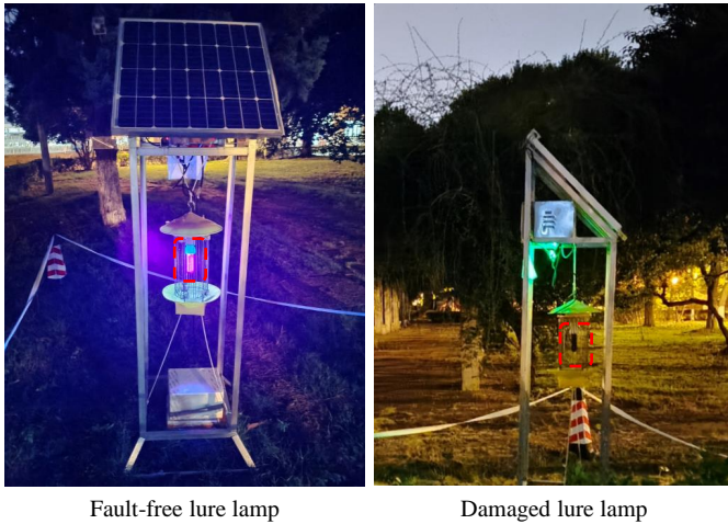
Fig. 6. The working conditions of the fault-free lure lamp and the damaged lure lamp at 11 p.m, where night mode is used to make photos bright at night.
