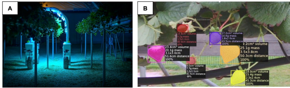
Fig. 3 A mobile robotic system equipped with an UVC light used for treating powdery mildew in strawberry developed by the partnership between Saga Robotics and University of Lincoln (photo by
