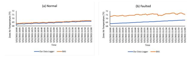
Figure 3: Zone temperature sensor faults identified as: (a) Normal; and (b) Faulted (bias)
