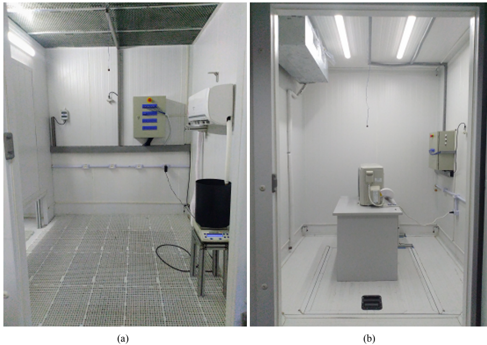
Figure 1: Calibrated calorimeter developed to evaluate the performance of the magnetocaloric air conditioner. (a) Indoor chamber, (b) outdoor chamber. The vapor compression evaporator and condensing unit shown in (a) and (b) were evaluated during the validation of the calorimeter.
