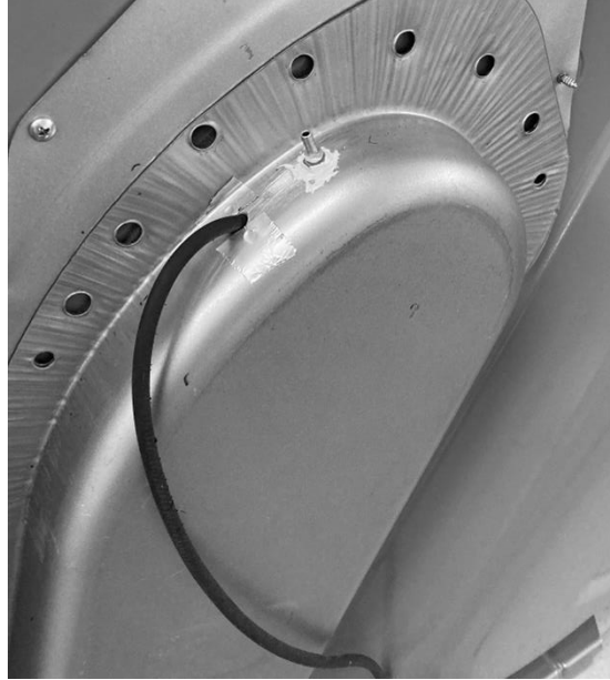
Figure 4: Photo of the rear duct, showing the locations of the two pressure taps for the Rear Grill Inlet and Rear Grill Out
