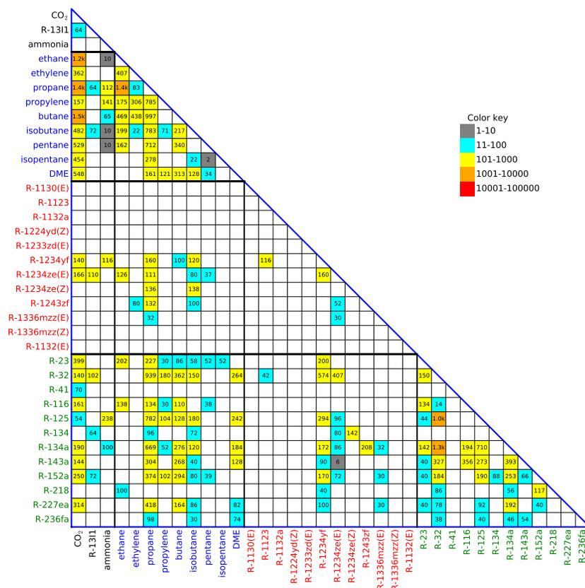
**Figure 1: VLE data coverage triangle.** An entry in a cell formed by a row and column label intersection indicates the total number of datapoints available in NIST TDE database (Diky et al., 2017) for this binary pair. Bubble-points and dew-points are counted separately. Figure reproduced from Bell et al. (2021).
