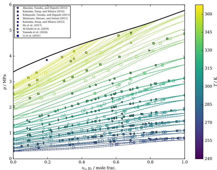
**Figure 6: Isothermal pressure-composition plot for R-32/1234yf with the new thermodynamic model and experimental data (Akasaka et al., 2013; Kamiaka et al., 2010; Kobayashi et al., 2011; Shimoura et al., 2011; Kamiaka et al., 2013; Hu et al., 2017; Al Ghafri et al., 2019; Yamada et al., 2020; Li et al., 2021). Filled markers are bubble points, open markers are dew points, the colored curves are isotherms, and the thick black curve is the critical curve.**
