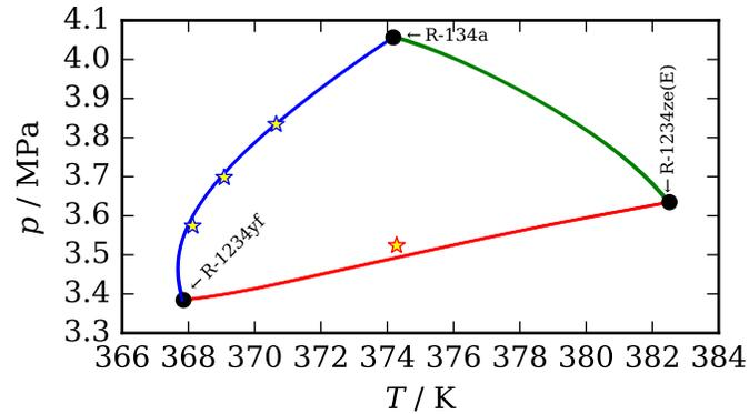
**Figure 2: Critical curves and experimental data (Akasaka et al., 2015; Higashi, 2016) for the three primary binary pairs; symbols indicate experimental datapoints and curves are model results traced with teqp (Bell et al., 2022; Deiters and Bell, 2020). Figure reproduced from Bell (2022).**
