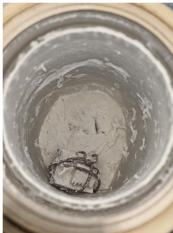
(b)CrMo + Brass + Al wire 22,23&24 6 weeks at 80 °C No oil/ 100 or 1000 ppm Air
