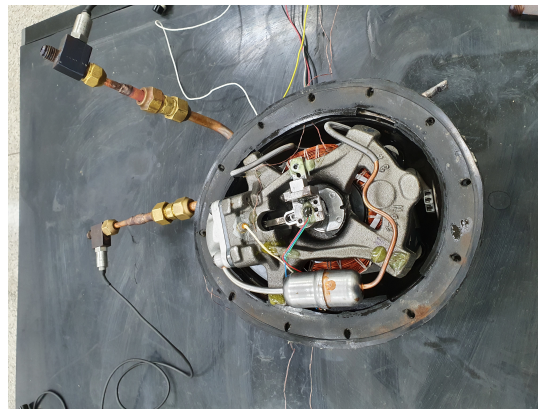
Figure 3: Instrumented compressor applied in start-up test
