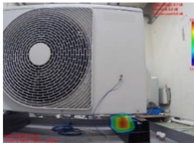
Figure 3: Beamforming map of the outdoor unit
