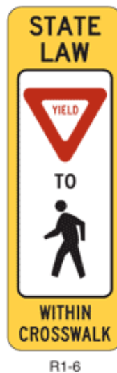
Figure 1 R1-6 Sign at Semi-Controlled Crosswalk
