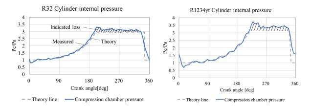
Figure 4: Internal pressure diagram of swing compressor
