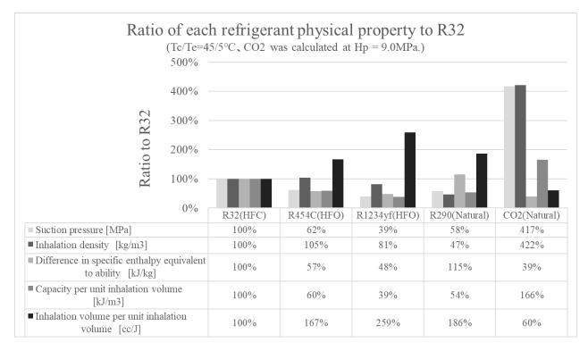
Figure 1: Ratio of each refrigerant physical property to R32
