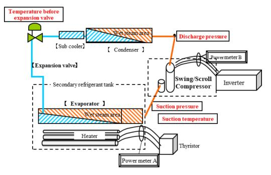
Figure 2: Test equipment: Calorimeter
