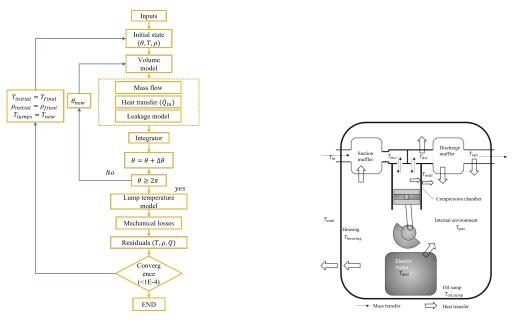
(a) Simplified model schematic for mechanistic chamber model-(b) Block diagram to represent various heat transfer phenomenon inside the compressor.
