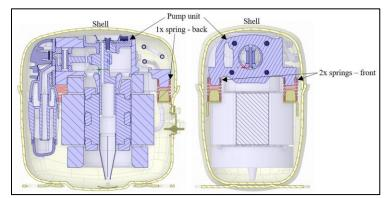
Figure 1: Schematic view: compressor with shell, pump unit and springs
