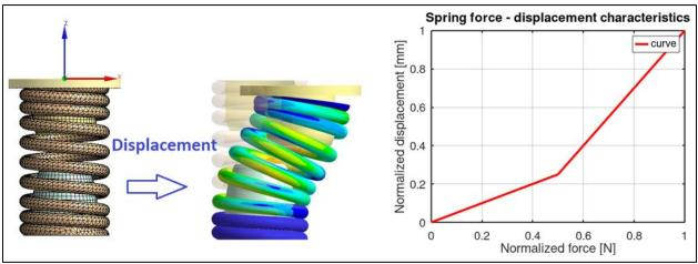
Figure 4: Force versus displacement function in a spring
