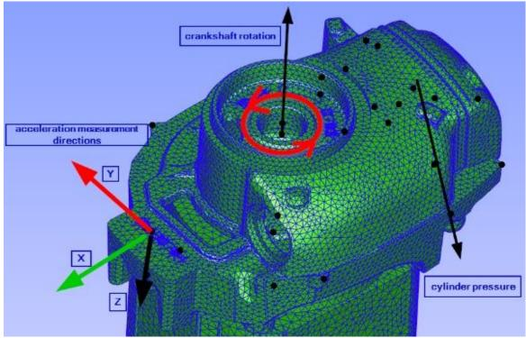
Figure 5: Experimental setup - measured characteristics
