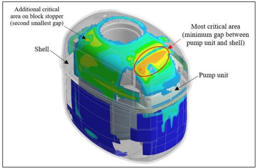
Figure 8: Minimum gap identification visualized
