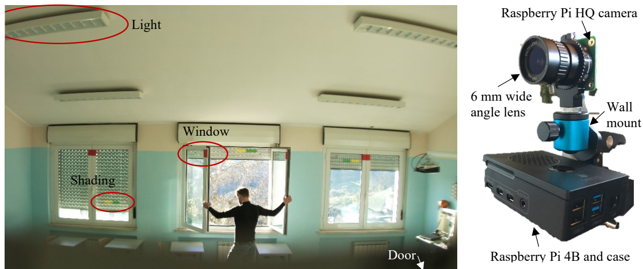
Figure 1: Camera perspective on classroom (left); Camera & Raspberry Pi setup (right)
