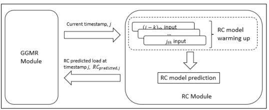
Figure 1 Underlying communication for hybrid approach.
