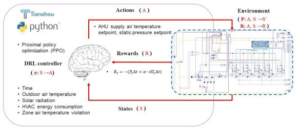
Figure 1: Schematics of DRLC formulation and implementation
