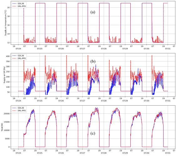
Figure 4: Time series of (a) SAT setpoint (b) static DP setpoint (c) Total HVAC power consumption during cooling season week for DRLC
