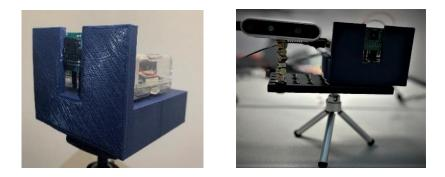
Figure 1: Thermal capture prototype (left) – Dual camera setup (right)
