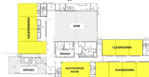
Figure 2: Plan view of the first floor (zones with convective system are highlighted)
