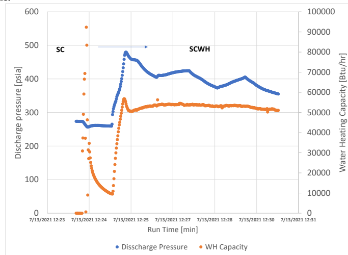
Figure 9: Mode Transition from SC mode to SCWH mode.
