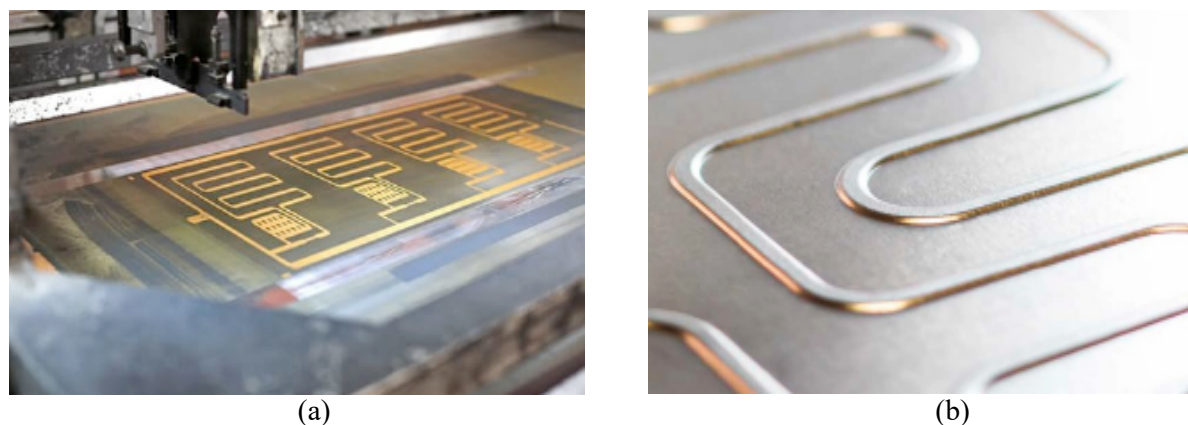
Figure 3: Roll-bond heat exchanger manufacturing process: (a) ink application before bonding process; (b) finished Roll-Bond Heat Exchanger.
