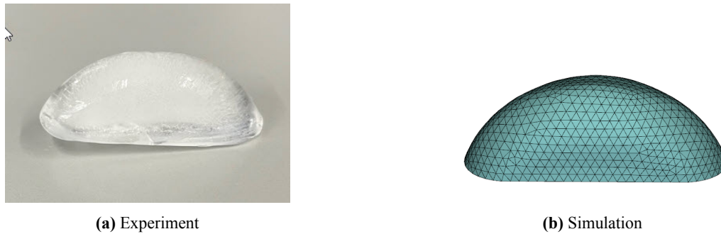
Figure 4: Ice particle – (a) Actual ice particle, (b) Simulation particle - 1271 facets.
