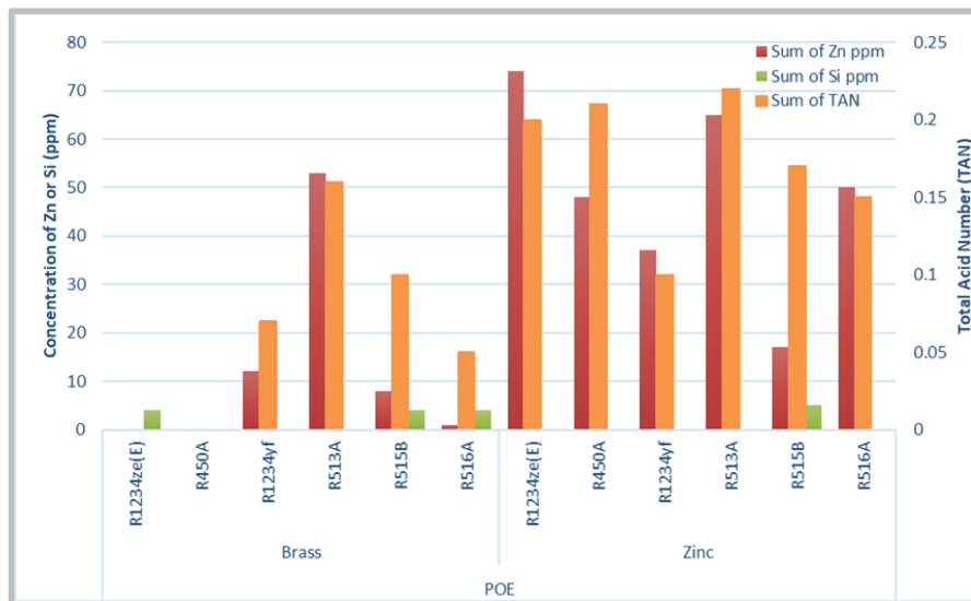
Figure 4: Summary of Dissolved Zinc, Silicon and TAN in POE Evaluations. Fluoride was not detected, so it is not shown.
