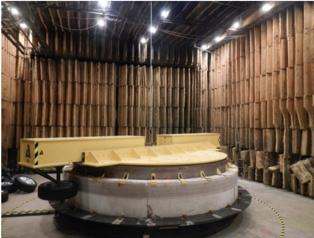
TPTA in hemi-anechoic chamber
