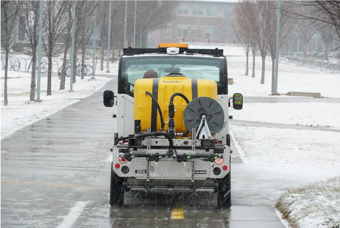
Figure 7. Precision brine prototype vehicle applying material at Purdue University.
