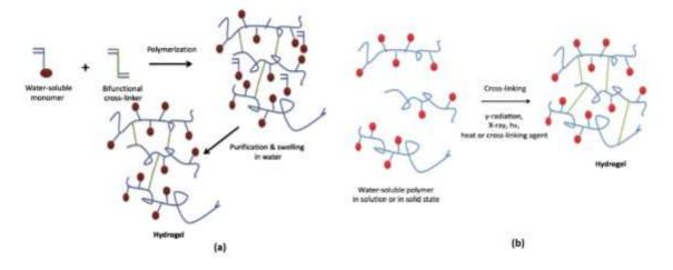
Figure 4. Classification of hydrogels based on the different properties [70]
