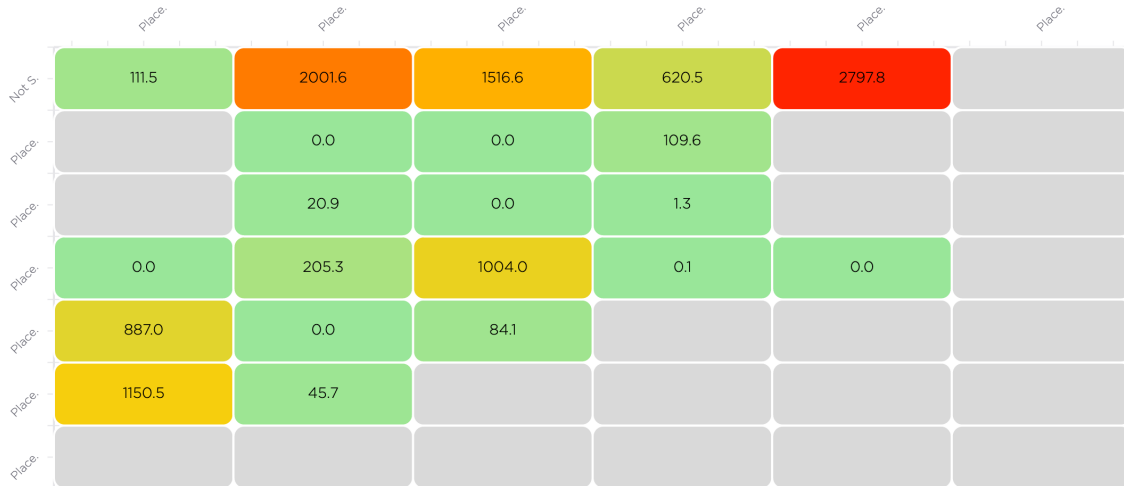
Figure 11: Heatmap for mean times in the production line queues.
