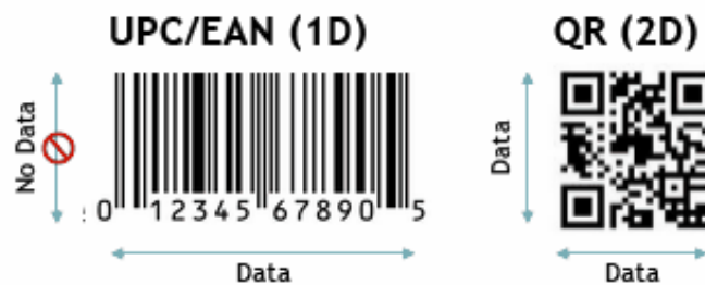
Figure 4: 1D vs 2D barcodes. [44]
