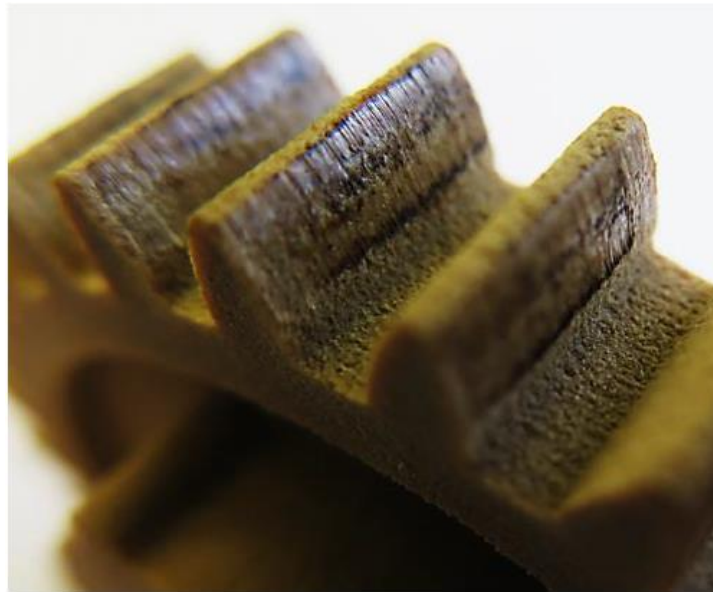
Figure 6.16: scuffing on addenda of gear tooth
