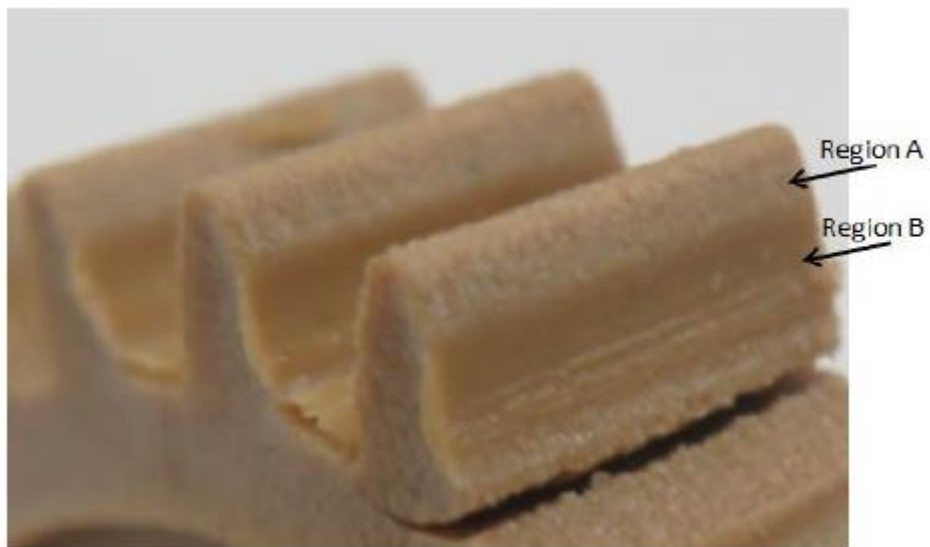
Figure 6.6: Regions of failure: Region A and Region B, surface fracture
