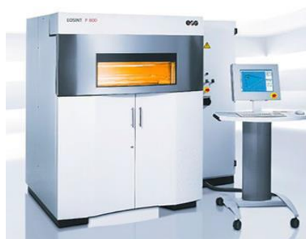
Figure 3.20: Electro Optical Systems (EOS) P800 High Temperature Laser Sintering (HTLS) system, (source EOS) 2
