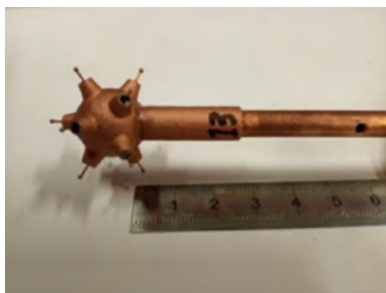
Figure 4.15: ACHINOS using an Araldite-copper layer on the 3-D-printed structure to form the central electrode.
