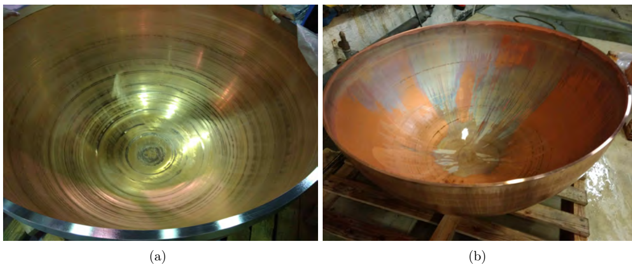
Figure 6.7: A detector hemisphere following (a) initial cleaning with detergent and (b) sanding and chemical etching with an acidified hydrogen peroxide solution. The discolouration observed in the latter is a result of oxidation of the copper and it is removed when the hemisphere is put in contact with the electrolyte.
