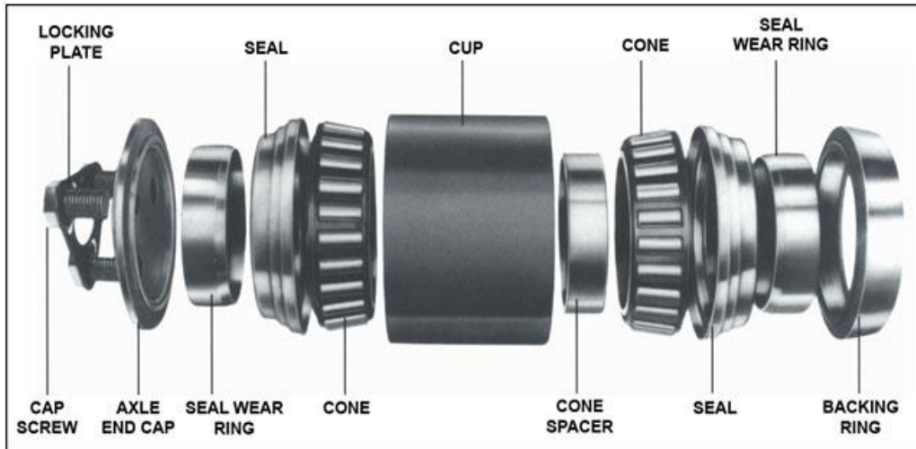
Figure 2-0-5: Schematic of a tapered roller bearing (Timken 2015)
