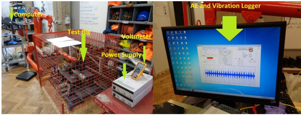
Figure 0-0-0-5: Customized bearing test rig 2 at the University of Birmingham. The photograph on the right shows the AE and Vibration data logger.
