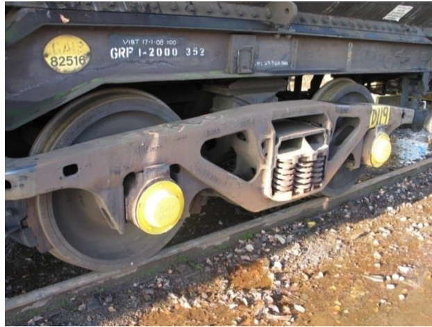
Figure 2-0-9: Photograph showing a typical bogie suspension
