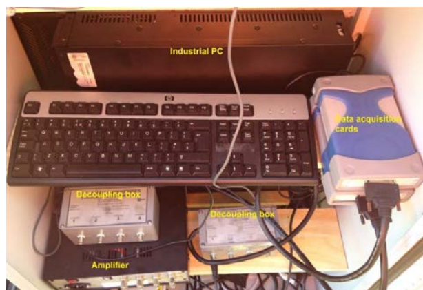
Figure 0-0-0-1: The customized data acquisition equipment used during laboratory and field trials (Amini 2016b)
