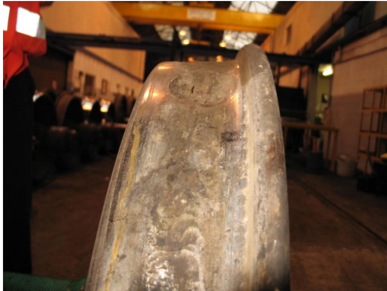
Figure 2-0-1: Photograph showing multiple wheel flats
