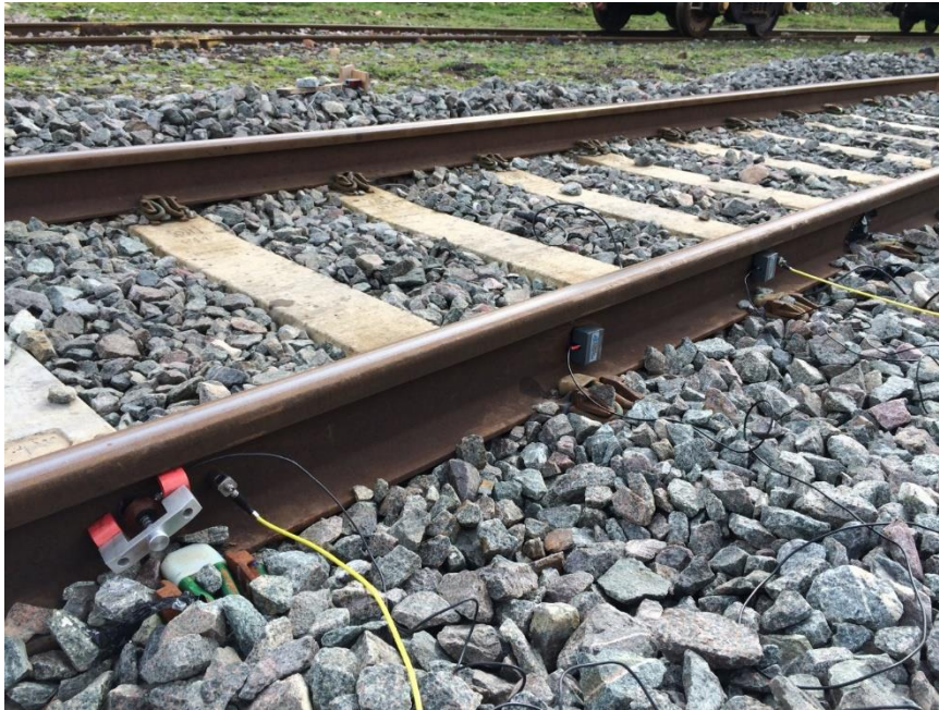
Figure 0-0-0-13: Photograph showing the AE sensors and accelerometers installed on the web rail at Long Marston, UK (Amini 2016b)
