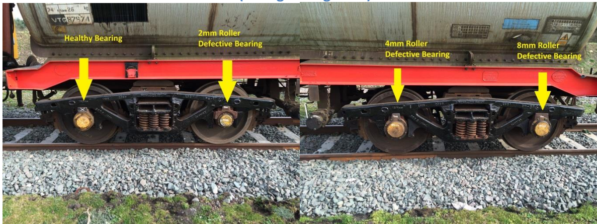
Figure 0-0-0-14: Schematic showing the experimental set-up with all the bearing defects (Zheng Huang 2017)
