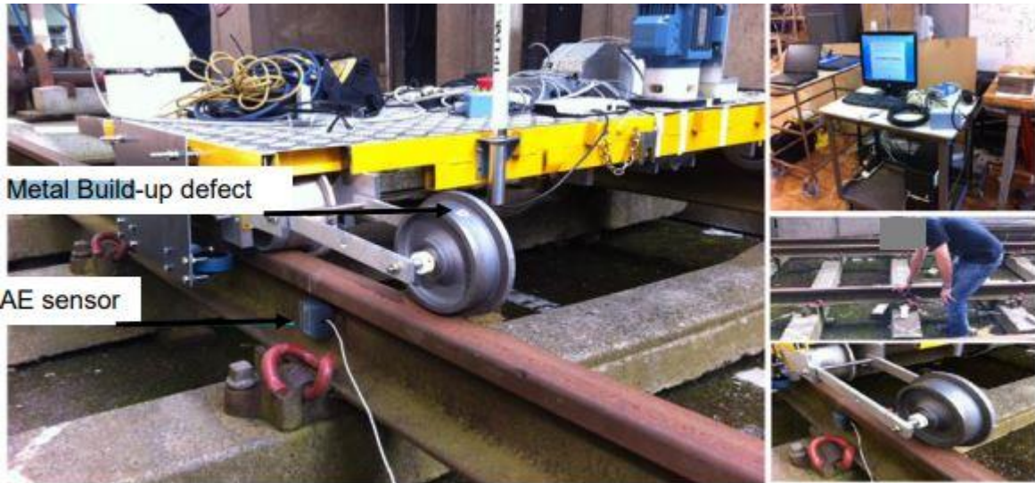
Figure 2-0-4 shows wheel with metal build- up defect during AE experiments at University of Birmingham (Amini et al. 2016a).
