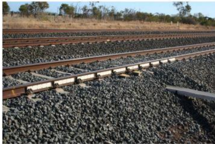
Figure 3-0-8: WILD based on strain gauges (photography courtesy of Markus Wong)
