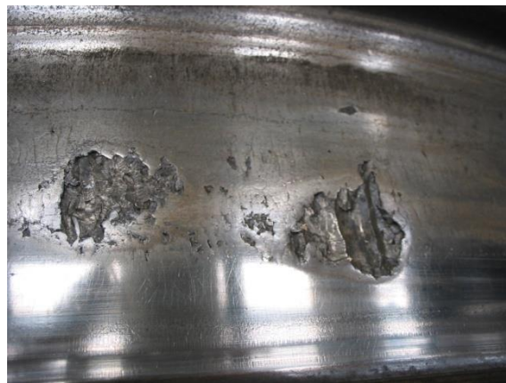
Figure 2-0-3: Photograph showing shelling on wheel tread (M. Papaelias et al. 2014b)
