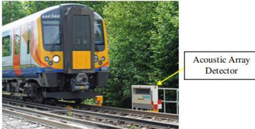
Figure 3-0-7: AADs trial in the UK network near London. The photography is courtesy of SIEMENS (M. Papaalias et al. 2014a)
