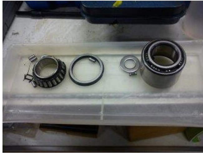
Figure 0-0-0-8: A rig double raw tapered roller bearing disassembled
