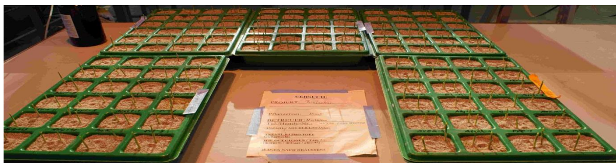
Figure 3-16 Completely randomized block design Exp_3; 20 treatments with 5 replicates blocked in racks
