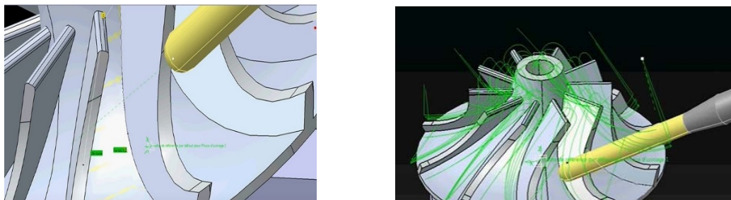
Figure 2.8 Finishing of the impeller root
