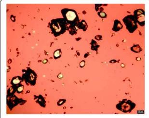
Fig. 2 Morphology of SP crystals
