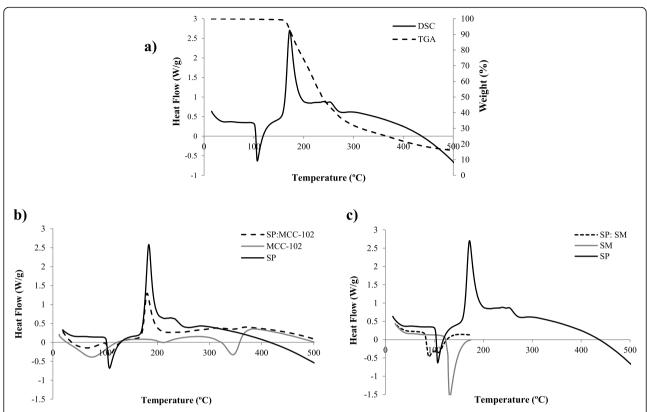
Fig. 5 Thermal analysis of SP, MCC-102, SM, and physical mixtures: a TGA and DSC curves of SP, **b** DSC thermograms of SP:MCC-102 (1:1) physical mixture and the pure materials, **c** DSC curves of SP:SM (1:1) physical mixture and the pure materials
