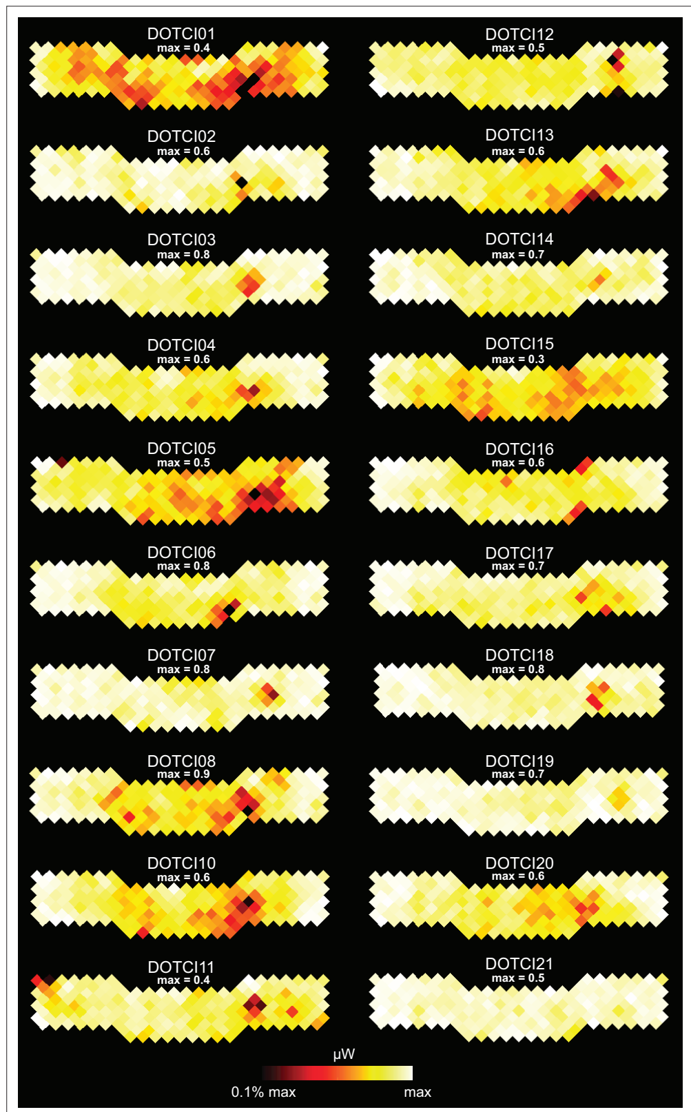
Figure 3—figure supplement 1. Coupling coefficients of each source and detector is shown in a flat view for all cochlear implant (CI) users included in the study. The dark red areas show the location of the signal drop for each CI user. The maximum coupling coefficient for each subject is shown above each plot.
