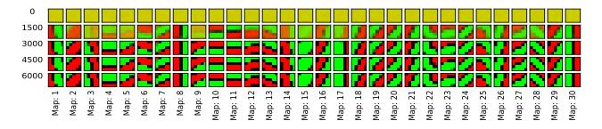
Fig. 5. Evolution of learned feature maps in the first convolution layer. Red and Green indicate ON and OFF center synapses respectively.
