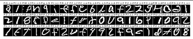
Fig. 10. Frequently misclassified classes in the EMNIST dataset. P and L denote predicted class and actual label, respectively.
