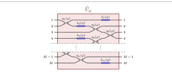
**Figure 1.** An M-mode passive linear interferometer composed of an arbitrary number of beam splitters and phase shifters having different and generic dependencies on a parameter  $\varphi$ . This scheme may represent for example the situation where  $\varphi$  is the temperature or the magnitude of an electromagnetic or a gravitational field affecting the optical properties of the interferometer components.
