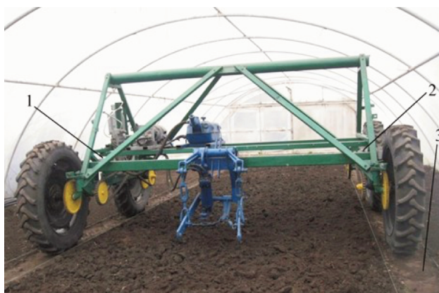
Figure 1. The wide span vehicle during the test: 1 - frame; 2 - electric motors; 3 - permanent traffic lanes.
