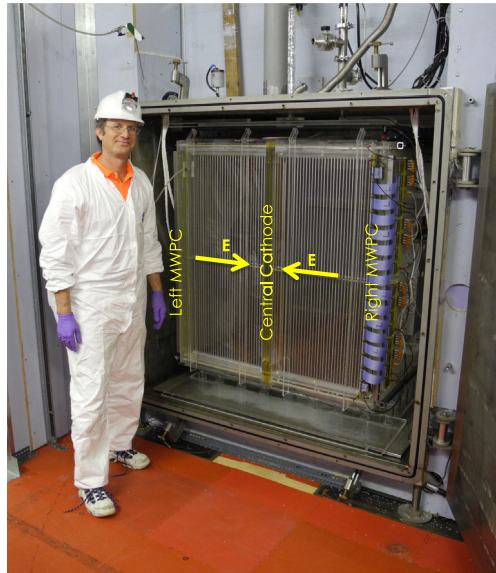
Fig. 3. The DRIFT-II detector in the Boulby Mine.
