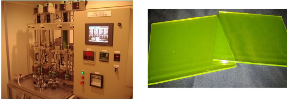
Fig. 22. Left: Self-production machine for nuclear emulsion gel. Right: NIT device coated onto a glass base.
