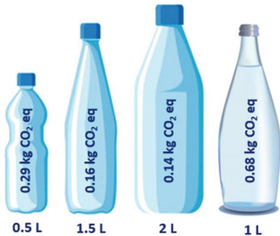
Fig. 7 Carbon footprint per material and size on average. Source Personal elaboration by EPD Vera [17], EPD Lete and Sorgesana [18], EPD Cerelia [19], EPD Levico [20] and EPD Frasassi [21]
