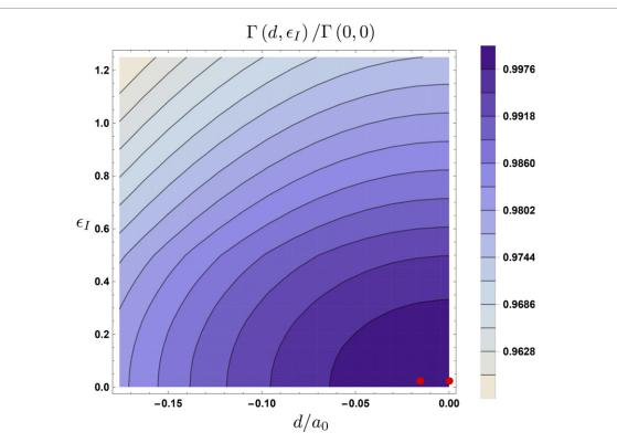
**Figure 7.** Ratio of the spontaneous emission rate  $\Gamma$  over the symmetric and non dispersive one  $\Gamma(0,0)$ , as a function of  $d/a_0$  and  $\epsilon_1$  and at fixed  $\epsilon_R = 11.638$ . The red dots represent the values of  $\Gamma$  mentioned in the text for the approximated QW at  $\epsilon_I = 0.024$  with d = 0 and  $d = -0.0153ea_0$ .
