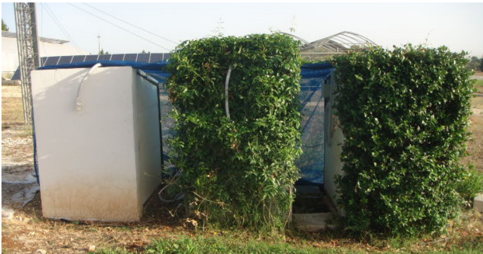
Figure 1: The three walls at the experimental field of the University of Bari: the uncovered control (the left wall), the Pandorea jasminoides variegated green façade (on the central wall), the Rhynchospermum jasminoides green façade (on the right wall).
