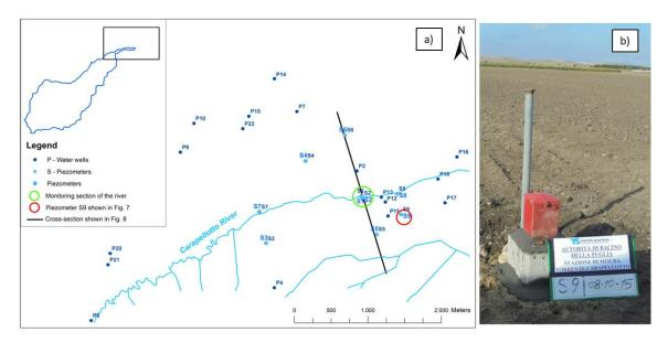
**Figure 6.** (a) Setting of the groundwater monitoring network. (b) Example of a groundwater monitoring well.
