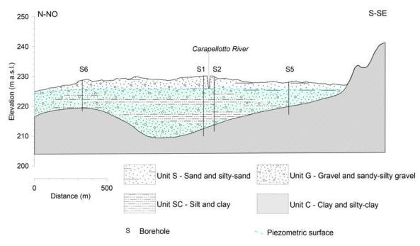
**Figure 7.** Hydro-stratigraphic cross-section along the monitored station in the Carapellotto river (location shown in Figure 6).
