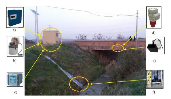
**Figure 3.** Monitoring station equipment: (**a**) modular transmitter; (**b**) automatic sampler; (**c**) turbidity probe controller; (**d**) ultrasonic level sensor; (**e**) optical velocity sensor; (**f**) turbidity probe, floating system and flow level gauge.
