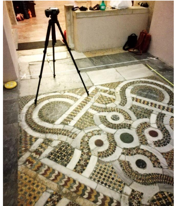
Figure 2. Photographic acquisition of mosaics in the crypt of the St. Nicola's Basilica in Bari
