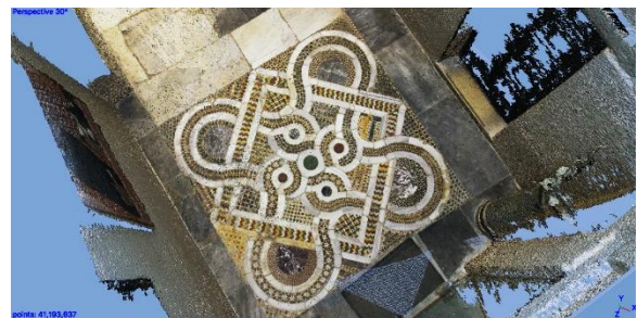
Figure 4. Digital 3D survey of the mosaic under the Catepan tower, St. Nicola's crypt, Bari
