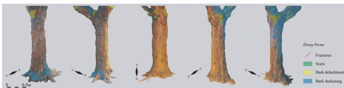
Figure 7. CRP 3D model of the studied living holm oak and shallow decay forms (2018 survey).
