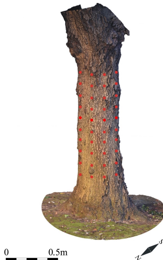
Figure 6. Ultrasonic measurement point locations in the 3D CRP model.
