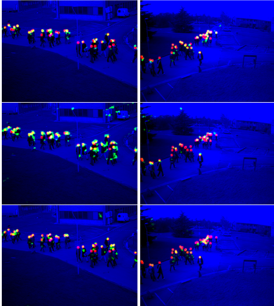
Figure 4.3: Density maps produced on two frames of PETSview1 (left) and PETSview2 (right) by the MCNN model trained on: synthetic images (top), the single-scene PETSview3 data set (middle), and the multi-scene ShanghaiTech PartB data set (bottom). The ground truth (red) and estimated (green) density maps are superimposed on the original frames. The yellow regions are the ones where the two maps coincide, corresponding to perfect localisation of pedestrians. The highest localisation accuracy is achieved when synthetic training images are used (top).
