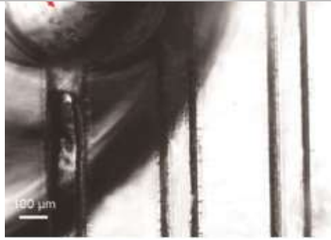
Fig. 5. This image shows the Jurkat cells that accumulated in a hole in the middle of the serpentine channel that was made intentionally in order to verify that this kind of cell does not adhere to the biofunctionalized channel's surface, but rather is dragged by microfluidic forces toward the additional outlet.
